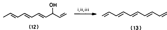
(only isomer) Reagents and conditions: i, PBr 3 ; ii, PhCH 2 NMe 2 ; iii, aq. NaOH, 100 °C
